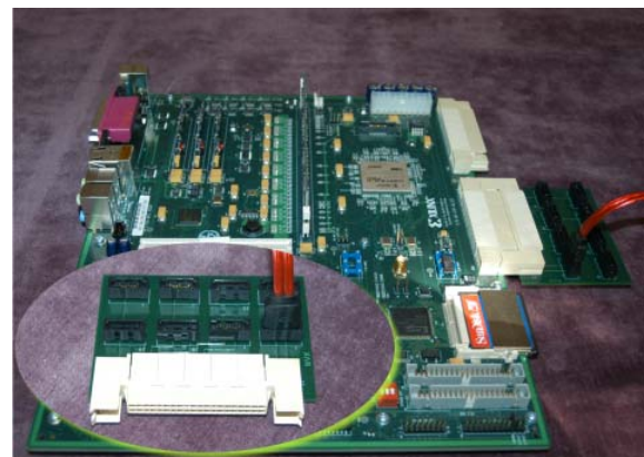
Figure 5. ML-310 with installed with our custom multi-gigabit transceivers to SATA adapter board (inset)
